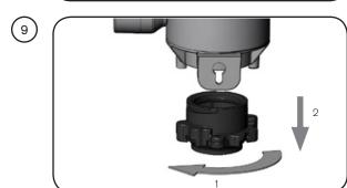
Ensure sleeve bolt is rotated full 1/4 turn until positive stop.
