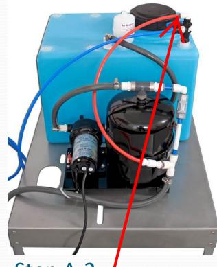
Step A-2 Insert Red Tubing in top Push-To-Connect on Divert Valve.
