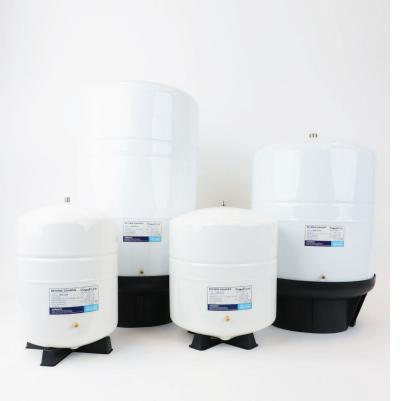
neoPure<sup>™</sup> Reverse Osmosis Tanks are built with FDA approved materials. The water storage chamber features a virgin polypropylene liner, high-grade chlorobutyl diaphragm and stainless steel water connection. The diaphragm is post cured to ensure that your water is tasteless, odorless and contaminant free. The tank is built with a sealed brass air valve and o-ring sealed cap to ensure a leak-free air chamber.
