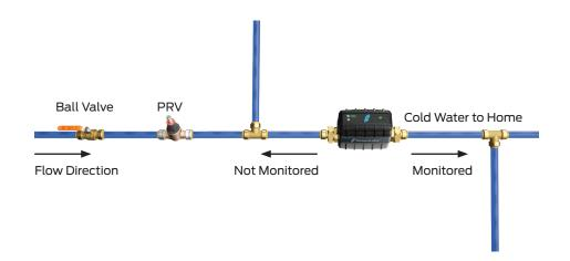
Take note to install the Control prior to any pipe branches. Branches prior to the Control will not be monitored or protected. At your installation location, you must have access to an electrical outlet and a Wi-Fi signal. The Control comes with a DC power adapter with a 10 foot cord. Power adapters of additional lengths can be purchased from StreamLabswater.com.
