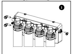
Connect quick connect elbows to the three open connection locations on the unit. Firmly push the fittings into place, then pull back lightly to lock them in.
