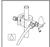
7. Once all lines are connected to the RO system turn on cold water supply. Turn Valve counter-clockwise and check for any leaks. Run water from the faucet to clear any debris caused by installation.
