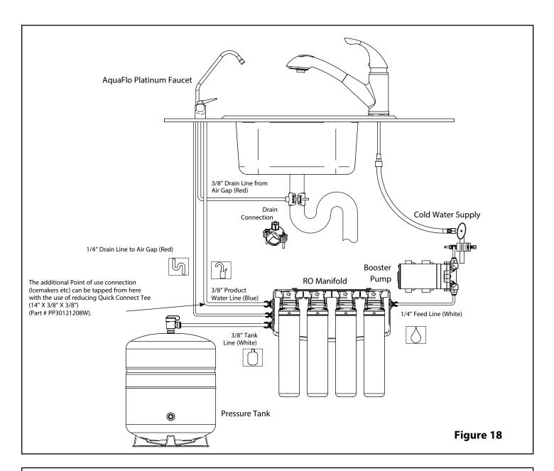
**ADDITIONAL POINT OF USE CONNECTION (Fittings and tubing for additional point of use connection is not supplied with this system) NOTE:** *Icemakers typically use 1/4" tubing as feed line.*
