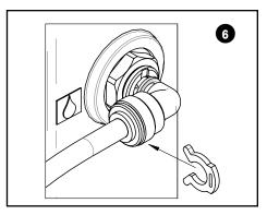
Attach locking clips to each white elbow fitting. Do not attach one to the blue flow control. Clips should slide in behind collet on the fittings.
