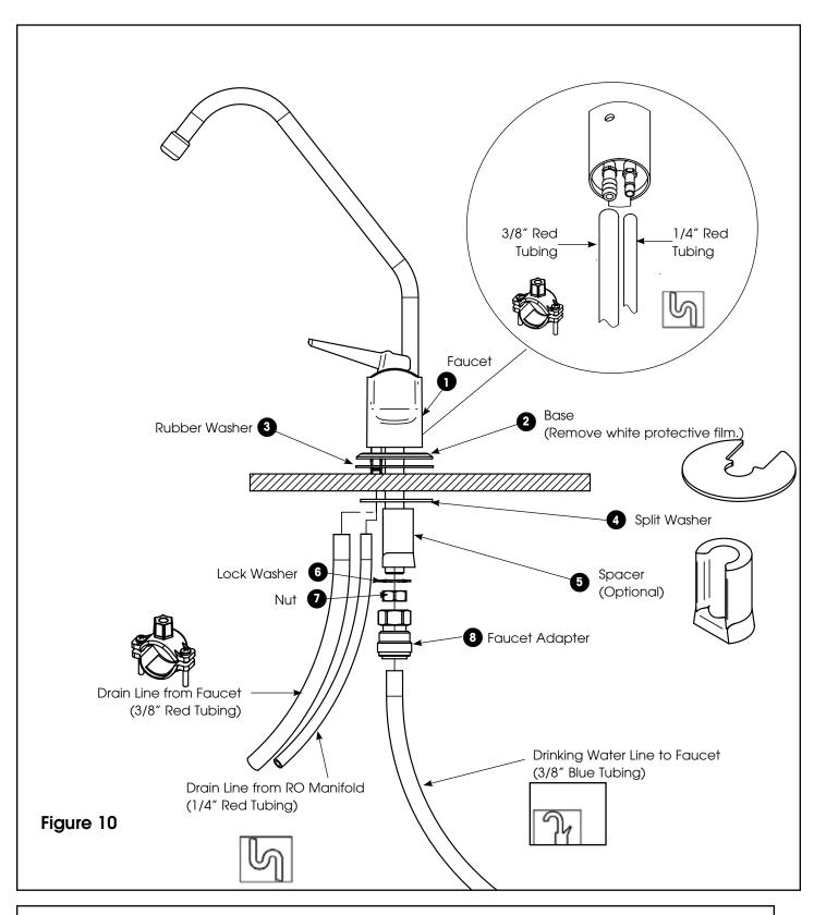
**NOTE:** The spacer is required for stainless steel sinks and thin counter tops. If sink is being installed on a thick (5/8" or thicker) counter the spacer is not required. Remove white protective film from faucet base.
