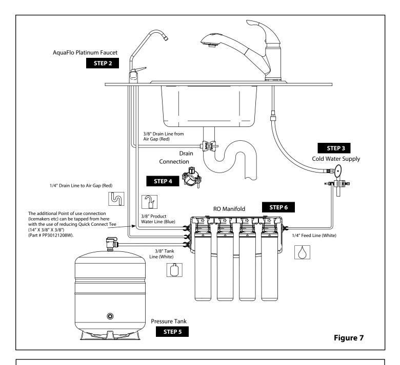
**NOTE:** Install the 3/8" red drain line from the air gap faucet to the drain adapter so that it runs downward with no loops or low spots. Otherwise the unit will overflow at the air gap siphon break built into the faucet, or make irritating gurgling sounds.
