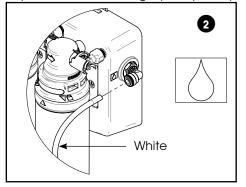
Connect 1/4-inch OD white plastic tubing from the feed water supply source to the system inlet on the manifold.
