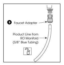
3. Take another length of 3/8" tubing and make sure it is has a fresh cut and is free of foreign materials and any scratches on the outside surface. Install the tubing into the push in type fitting at the base of the faucet. Make certain that it is inserted all the way in; once inserted give it a slight pull to make sure it is locked into the fitting. You have now completed the tubing connections.
