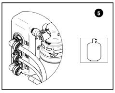
Connect the 3/8" OD white product water tube from the tank to the manifold.
