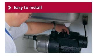
The Grundfos' MQ pump is compact and extremely easy to install. The pressure switch and tank are already built into the MQ. Furthermore, it is selfpriming and water-cooled with a very low noise level. The outlet pipe connection can be angled up to 5° to fit your existing pipe-work.
