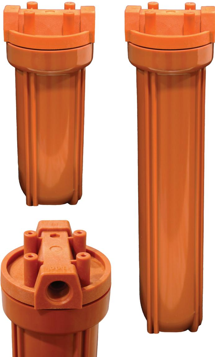
neoPure High Temperature Standard Filter Housings are manufactured of a Glass Reinforced Nylon. Available with 3/4 NPT ports. Housings are available in 10" and 20" lengths and will accommodate a wide range of 2-1/2" to 2-7/8" diameter cartridges.
