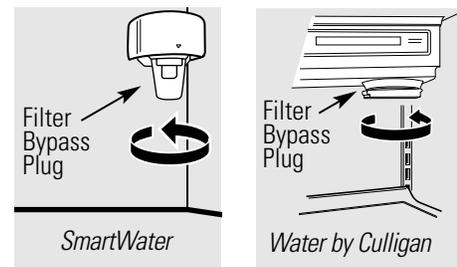
To use the filter bypass plug on *Water by Culligan* models, you must first remove the filter adapter from the cartridge holder by turning it to the left.
