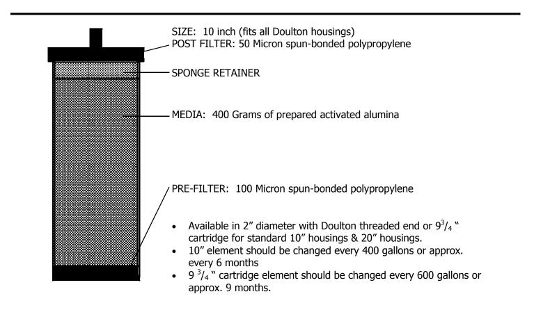
• The A-2 element has also been shown to reduce arsenic to less than 0.02 ppm from 0.12 ppm in the supply water. Total capacity for arsenic has not been determined.
