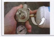
STEP 16 (Exubera only) – Set the sparkling water out-flow on the flow compensator (clear transparent box connected to the faucet tubing) to ensure you dispense 1/4 gallon of sparkling water in about 35 seconds. If needed: adjust the flow in this manner: clockwise decreases flow, counter clockwise increases flow.
