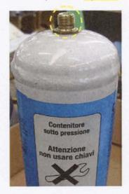
Using just your hands (do not tighten with wrench!), screw the CO2 cylinder to the pressure reducer gauge until you seal it (do not over tighten). Make sure the pressure gauge is set between 45-60 psi (3-4 bar).
