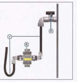
STEP 7 – Install in the tube from step 6 the water PRV (Pressure Reducing Valve) R, included with the installation kit, according to the water flow marked on it. This needs to be installed if your main water pressure exceeds 43.5psi.
