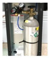
10. Replace door and drip tray. Dispense a few cups of carbonated water to allow initial mix of water & CO2 Gas. Allow water sufficient time to chill before ideal carbonation. Four to five hours is recommended after the initial set-up.
