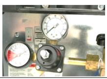
7. Purge air from Carbonator by simultaneously pulling the Ring Pull on the safety valve while pressing the CO2 water button until water comes out of the valve. The ring is located inside the compartment at the top right near the CO2 cylinder.
