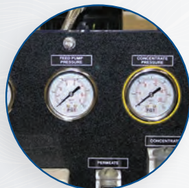
Liquid Filled Panel Mounted Concentrate Pressure Gauge
