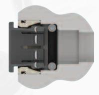
A collet or gripper made of acetal copolymer with stainless steel teeth to grip the tube.  A Body in food grade acetal, with stainless steel teeth that will grip into the housing of the equipment. **3.** An 'O' ring made from food grade material.
