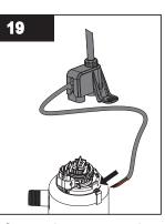
• Connect the green ground wire and red strain relief wire to the chamber using the grounding screw.
