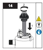
Insert and secure the lamp/ sleeve assembly.
