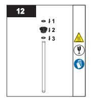
Insert new O-rings and tighten the sleeve bolt to the quartz sleeve.
