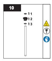
• Unscrew the sleeve bolt and remove O-rings from the quartz sleeve.
