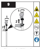
• Unscrew the UV lamp by holding the sleeve bolt.
