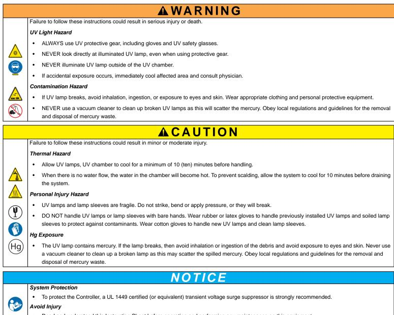
• Read and understand this Instruction Sheet before operating and performing any maintenance on this equipment.
