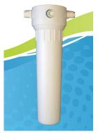
This is an in-line pressure filter housing molded from ABS and is supplied with the mounting bracket & screws. The inlet & outlet are 3/8" push-fit connectors for easy installation. Also available with a DIY installation kit which includes most parts needed for installation, including a faucet. This system is designed for cold water use only.
