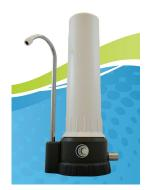
The HCP is a freestanding filter system for countertop use, which is readily attached to an existing faucet via a diverter valve. Housing is molded from acetal and polyester materials. This system needs no permanent modifications to the plumbing. The system allows filtered or unfiltered water to be drawn from the existing faucet. This system is designed for cold water use only.
