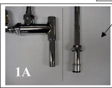
Step 1A: Remove Riser from Base Faucet by unthreading Easy Install locking nut and pulling up until the riser "pops" out.
