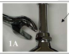
**Step 1A:** Loosen the Easy Install locking nut from the riser to base-faucet connection.
